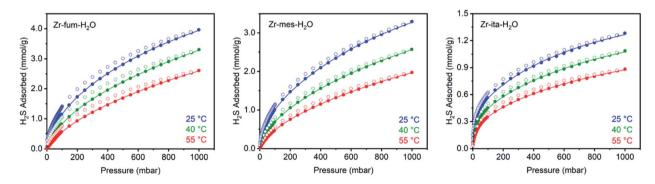
Fig. 3  $H_2S$  adsorption (closed circles) and desorption (open circles) isotherms at 25 °C (blue), 40 °C (green), and 55 °C (red) of activated Zr-fum- $H_2O$ , Zr-mes- $H_2O$ , and Zr-ita- $H_2O$ . Solid lines represent fits of the adsorption data to a Langmuir-Freundlich model. A data point was considered equilibrated after <0.01% pressure change occurred over a 45 s interval.
