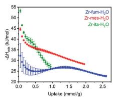
Fig. 4 Differential enthalpies of adsorption ( $-\Delta H_{ads}$ ) for  $H_2S$  as a function of uptake for activated Zr-fum- $H_2O$  (blue), Zr-mes- $H_2O$  (red), and Zr-ita- $H_2O$  (green), as determined using the Clausius-Clapeyron equation (eqn (1)) and Langmuir-Freundlich fits in Fig. 3. A data point was considered equilibrated after <0.01% pressure change occurred over a 45 s interval.
