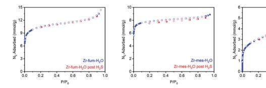
Fig. 5 77 K  $N_2$  adsorption isotherms of activated Zr-fum- $H_2O$ , Zr-mes- $H_2O$ , and Zr-ita- $H_2O$  before (blue) and after treatment with  $H_2S$  at 25 °C (red). After  $H_2S$  adsorption, the MOFs were regenerated at 100 °C under vacuum (<10  $\mu$ bar) for 48 h.
