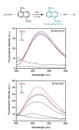
Fig. 9 Fluorescence assay (excitation at 340 nm) using the turn-on fluorescence probe dansyl azide (DNS-az) to confirm the release of  $H_2S$  from Zr-fum- $H_2O$  (upper) and Zr-ita- $H_2O$  (lower) upon submersion in phosphate buffered saline (PBS). The black line corresponds to a control experiment lacking MOF. The data were smoothed by adjacent-averaging (15 points).
