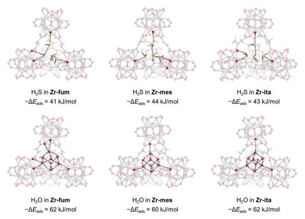
Fig. 7 DFT-calculated structures of  $H_2S$  binding in Zr-fum, Zr-mes, and Zr-ita with calculated energies of adsorption ( $-\Delta E_{ads}$ ) indicated. The DFT-calculated structures and energies of H<sub>2</sub>O adsorption in all three MOFs are included for comparison. Gray, white, red, yellow, and pale blue spheres correspond to carbon, hydrogen, oxygen, sulfur, and zirconium, respectively.
