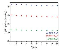
Fig. 6 Cycling capacities for  $H_2S$  adsorption (1 bar, 30 °C) in Zr-fum- $H_2O$ , Zr-mes- $H_2O$ , and Zr-ita- $H_2O$ . The samples were regenerated at 100 °C under high vacuum (<10  $\mu$ bar) between cycles.
