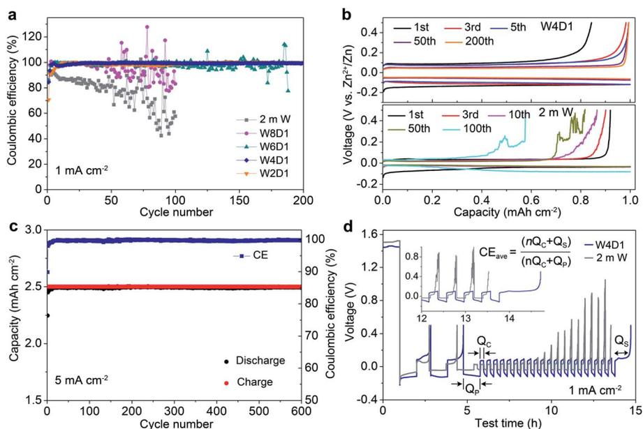
Fig. 3 Zn<sup>2+</sup> plating/stripping behaviors in H<sub>2</sub>O + DMC electrolytes. (a) Zn plating/stripping CE values of Zn/Ti cells in different electrolytes. (b) Typical voltage profiles of Zn/Ti cells in W4D1 and 2 m W at 1 mA cm<sup>-2</sup>. (c) Cycling stability and Zn plating/stripping CE of the Zn/Ti cell in W4D1 at 5 mA cm<sup>-2</sup>. (d) Evolution of voltage profiles of Zn/Ti cells in W4D1 and 2 m W electrolytes under a 'reservoir half-cell' method.
