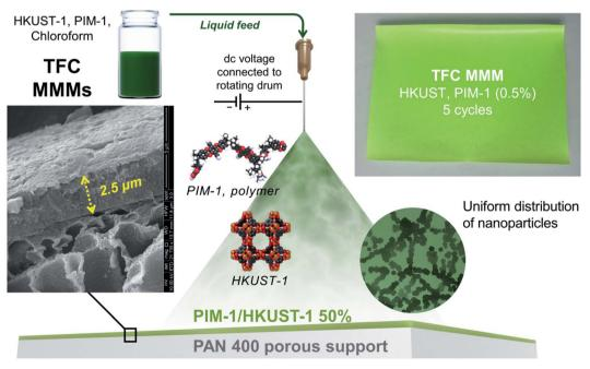
Fig. 1 Schematic demonstration of the electrospray 3D printing approach.
