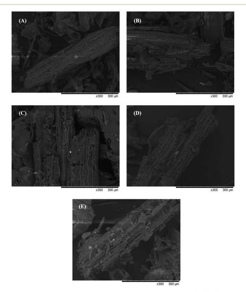
Fig. 2 Scanning electron microscope images of the microwave pretreated corn straw and the control. CK (A);  $120 \,^{\circ}$ C,  $10 \,^{\circ}$ C,
