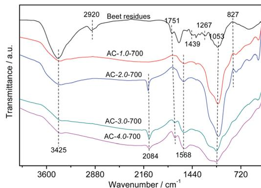
Fig. 5 FTIR spectra of the beet residue and AC samples.
