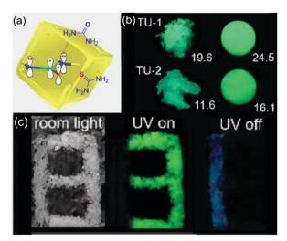
Fig. 25 (a) Structures of urea and TU and their delocalized  $\pi_6^4$  system. (b) Photographs of TU-1, TU-2, and their tablets taken under 312 nm UV light.  $\Phi$  values (%) of the samples are also given. (c) Pattern "8" comprising urea (blue part) and TU-1 (green part) crystals taken under room light, 312 nm UV light, and after ceasing the UV irradiation. Reprinted with permission from ref. 40. Copyright 2020, John Wiley and Sons.
