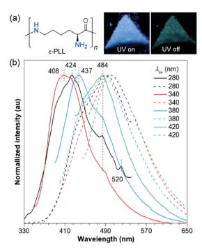
Fig. 22 (a) Structure of  $\varepsilon$ -PLL and the photograph of its powders taken under 365 nm UV light or after ceasing the irradiation. (b) Normalized emission spectra of  $\varepsilon$ -PLL powders with  $t_d$  of 0 (solid line) and 0.1 ms (dash line) under varying  $\lambda_{\text{ex}}$ . Reprinted with permission from ref. 89. Copyright 2018, Springer.
