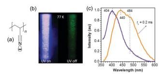
Fig. 19 (a) Structure of PAN. (b) Photographs of PAN powders taken at 77 K under 365 nm UV light or after ceasing the UV irradiation. (c) Emission spectra of PAN powders with  $t_d$  of 0 and 0.2 ms ( $\lambda_{ex}$  = 335 nm). Reprinted with permission from ref. 39. Copyright 2016, John Wiley and Sons.
