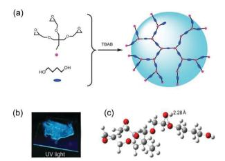
Fig. 9 (a) Schematic representation of the synthetic route for EHBPE. (b) Images of EHBPE in bulk under UV irradiation. (c) Optimized conformation of P1. Reprinted with permission from ref. 48. Copyright 2016, Royal Society of
