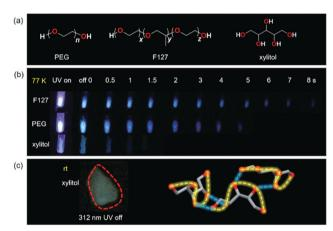
Fig. 21 (a) Structures of PEG, F127, and xylitol. (b) Photographs of the solid powders of F127, PEG, and xylitol taken under 312 nm UV light or after ceasing the UV irradiation at 77 K. (c) Photograph of xylitol powders taken at room temperature after ceasing the 312 nm UV irradiation, and partial electronic channels of O···O short contacts in xylitol crystals. Reprinted with permission from ref. 47. Copyright 2018, John Wiley and Sons.
