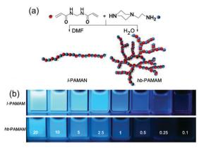
Fig. 3 (a) Synthetic route to linear (I) and hyperbranched (hb) PAMAMs. (b) Photographs taken under UV irradiation of aqueous solutions of I-PAMAM and hb-PAMAM at different concentrations. Reprinted with permission from ref. 22. Copyright 2015, Springer.
