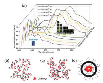
Fig. 20 (a) Steady-state PL and long-phosphorescence spectra of PU1 with different average molecular weights ( $M_n = 2672 \text{ or } 3118 \text{ g mol}^{-1}$ ) and different concentrations in 2-MeTHF solutions at 77 K. And schematic illustration of PU1 (b) dilute solution, (c) concentrated solution, and (d) carbonyl clusters in the aggregated state. Reprinted with permission from ref. 88. Copyright 2018, American Chemical Society.
