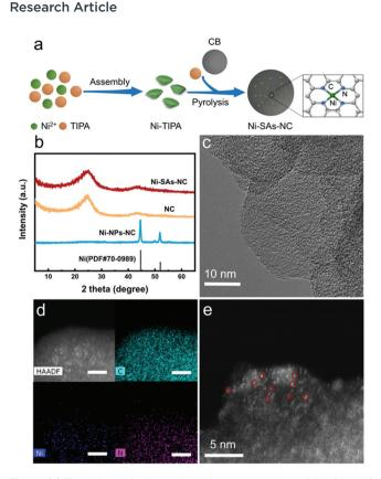
Fig. 1 (a) The schematic illustration of the preparation of Ni-SAs-NC. (b) PXRD patterns of Ni-SAs-NC, Ni-NPs-NC and NC. (c) TEM and (d) EDX elemental mapping images of Ni, C and N elements of Ni-SAs-NC (scale bar = 5 nm). (e) HAADF-STEM image of Ni-SAs-NC.
