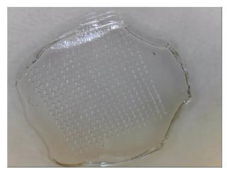
Fig. 4 CMC-MAL microneedle array structure consisting of 324 needles of height 750 μm, base diameter 200 μm, tip diameter 10 μm and centreto-centre spacing of 600 µm.
