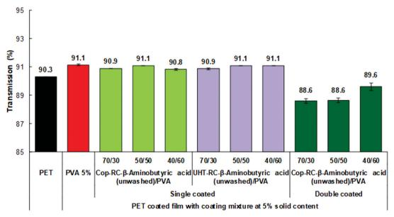
Fig. 4 Optical transmission of the coated films with Cop-RC-β aminobutyric acid at different ratios with a 5 wt% solid content.
