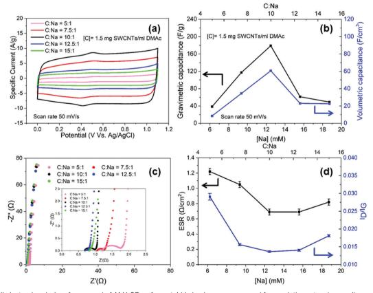
Fig. 2 Half-cell electrochemical performance, in 1 M H<sub>2</sub>SO<sub>4</sub>, of nanotubide buckypapers prepared from solutions at a given sodium concentration, or equivalent C: Na ratio: (a) CV curves at 50 mV s $^{-1}$ ; (b) gravimetric and volumetric capacitance of (a) normalised to the mass and volume of active electrode; (c) Nyquist plots and (d) ESR and the  $I_D$  to  $I_G$  ratio derived from Raman spectra.
