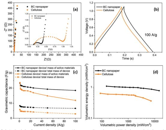
Fig. 4 Full-cell electrochemical performance of aqueous symmetric supercapacitors using nanotubide buckypaper electrodes sandwiched with BC nanopaper (black) and cellulose (orange) as separators: (a) Nyquist plots and (b) GCD curves at 100 A  $g^{-1}$ , (c) the calculated gravimetric capacitance normalised by both active material (straight line) and total mass of device (dash line) and (d) volumetric Ragone plots normalised by total mass of device.
