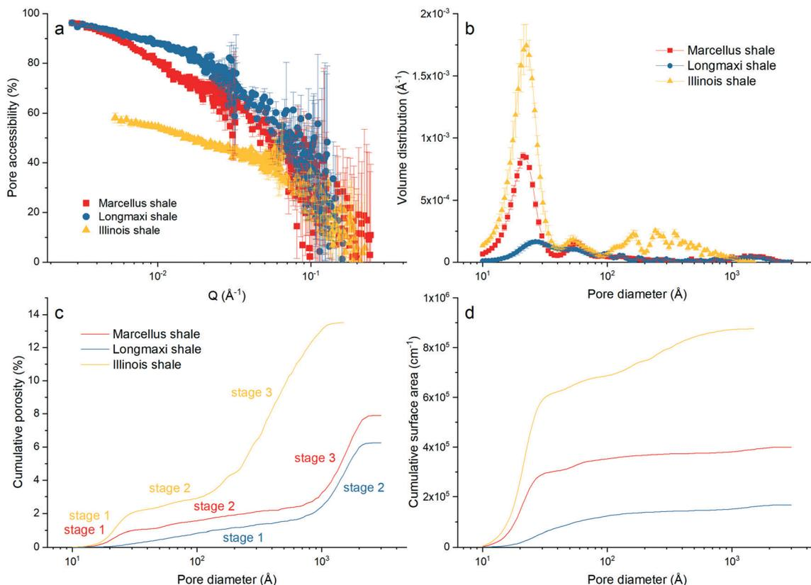
Fig. 3 (a) Pore accessibility, (b) pore volume distribution, and cumulative (c) porosity and (d) surface area of the three shale samples.
