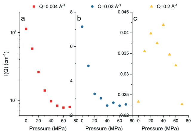
Fig. 2 Scattering intensity as a function of methane pressure at (a)  $Q$  of  $0.004 \text{ \AA}^{-1}$ , (b)  $Q$  of  $0.03 \text{ \AA}^{-1}$ , and (c)  $Q$  of  $0.2 \text{ \AA}^{-1}$  for the Marcellus shale sample.
