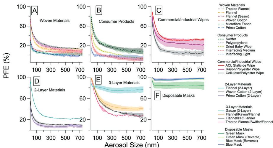
**Fig. 3** PFE as a function of aerosol size for all tested materials and multi-layer combinations, grouped according to material class: (A) woven materials; (B) consumer products; (C) commercial/industrial wipes; (D) 2-layer materials; (E) 3-layer materials; and (F) disposable masks. Variability shown is one standard deviation of the mean for the three tests.
