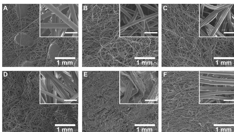
Fig. 1 SEM images of non-woven materials: (A) polypropylene; (B) Swiffer; (C) baby wipe; (D) rayon/polyester wipe; (E) cellulose/polyester wipe; (F) ACL staticide wipe. Scale bar in inset: 50  $\mu\text{m}$ .
