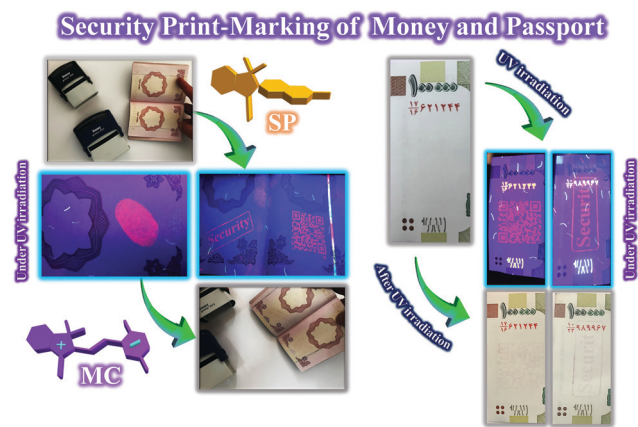
Fig. 11 Security print-marking on money and passport using different stamps loaded with the photochromic and fluorescent anticounterfeiting ink based on PMMA-SP.
