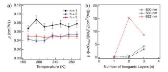
Fig. 6 Conductivities in layered hybrid perovskite powders and thin films based on  $A_2FA_{n-1}Pb_nI_{3n+1}$  perovskite with different compositions (n = 1-3). (a) Evolution of mobilities in powders at various temperatures and (b) conductivities in thin films deposited on quartz substrates at ambient temperature (298 K). The initial charge carrier concentration was estimated to be  $10^{14}$  to  $10^{16}$  cm<sup>-3</sup> at 298 K.
