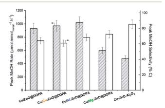
Fig. 4 Peak methanol rates and selectivity for the colloidal Cu/ZnO@DOPA, Cu/M:ZnO@DOPA catalysts and reference catalyst Cu–ZnO–Al $_2$ O $_3$  in the hydrogenation of CO $_2$  to methanol. Reaction conditions: 210 °C, 50 bar, CO $_2$ : H2 = 1:3, 150 mL min $^{-1}$ .
