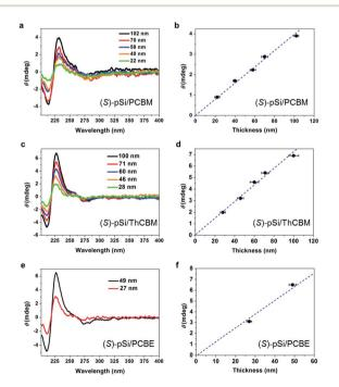
Fig. 7 CD spectra of (a) (S)-pSi/PCBM, (c) (S)-pSi/ThCBM, and (e) (S)-pSi/PCBE films with different thicknesses. Ellipticity of the positive peak at 230 nm in the CD spectra of (b) (S)-pSi/PCBM, (d) (S)-pSi/ThCBM, and (f) (S)-pSi/PCBE films plotted as a function of the film thickness. Dashed lines are the linear regressions of the data.
