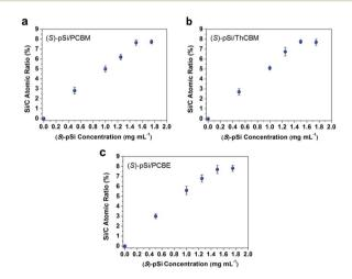
Fig. 3 Si/C atomic ratios on the surfaces of (a) (S)-pSi/PCBM, (b) (S)pSi/ThCBM, and (c) (S)-pSi/PCBE films plotted as a function of the (S)pSi concentrations in the blend solutions. The concentrations of PCBM, ThCBM, and PCBE were fixed at 10 mg  $\,\mathrm{mL^{-1}}$ . All the films were spin-coated on silicon wafers, and then annealed at 150 °C for 30 min before XPS measurements
