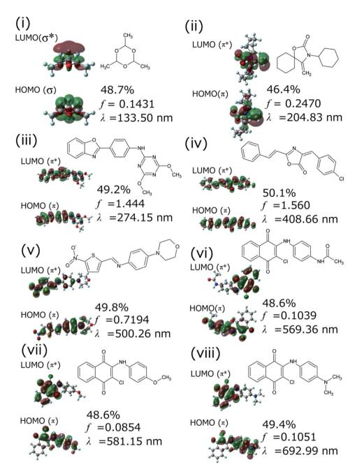
Fig. 5 Dominant electronic transition (given as a percentage) to the first excited ( $S_1$ ) state of selected molecules (i)–(viii) found by BLOX as calculated by quantum chemical calculations at the B3LYP/6-31G\* level. All the  $S_1$  states are attributed to a HOMO–LUMO single electron transition. f and  $\lambda$  are the oscillator strength and the wavelength, respectively.
