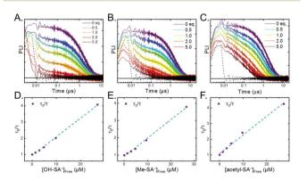
Fig. 7 A–C) Time-resolved photoluminescence decays for Ru-Bpz (25  $\mu$ M) upon the addition of up to 5 equivalents of (A and D) OH-SA<sup>-</sup>, (B and E) Me-SA<sup>-</sup>, (C and F) acetyl-SA<sup>-</sup>. Black dotted lines are the instrument response function based on a scattered laser pulse with no sample present. (D–F) Dynamic Stern–Volmer plots. Blue dashed line is a linear fit to the data.
