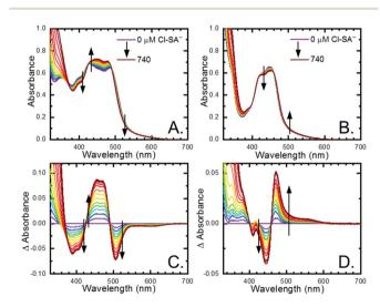
Fig. 4 UV-visible absorption spectra of (A) Ru-Dtb and (B) Ru-Bpz ( $\sim$ 25  $\mu$ M) upon the addition of 0 to 740  $\mu$ M Cl-SA<sup>-</sup>. Difference spectra calculated by subtracting the absorption spectra at no Cl-SA<sup>-</sup> from the spectra with Cl-SA<sup>-</sup> present for (C) Ru-Dtb and (D) Ru-Bpz. Arrows indicate the spectral changes upon Cl-SA<sup>-</sup> addition.
