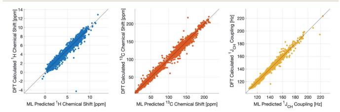
Fig. 2 IMPRESSION machine learning predictions compared to DFT computed NMR parameters for  $\delta^1$ H (left),  $\delta^{13}$ C (centre) and  $^1J_{CH}$  couplings (right) without variance filtering.
