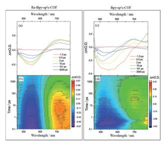
Fig. 4 Transient absorption spectra of (a) Re-Bpy-sp<sup>2</sup>c-COF and (c) Bpy-sp<sup>2</sup>c-COF at pump-probe time delays chosen to highlight the changing nature of the excited electronic states probed, and the complete transient absorption surface probed (b) Re-Bpy-sp<sup>2</sup>c-COF and (d) Bpy-sp<sup>2</sup>c-COF. All spectra are recorded in CH<sub>3</sub>CN following 400 nm excitation.
