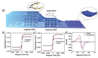
Fig. 6 Anisotropy of magnetic properties in ordered NW films. (a) Schematic illustration of the magnetic assembly process. (b) The magnetization of the ordered NW film with the magnetic field parallel and perpendicular to the orientation. The EPR spectra of the aligned (c) and random (d) sample in the parallel and perpendicular direction. (a-d) Reprinted with permission from ref. 84. Copyright 2020 Wiley.
