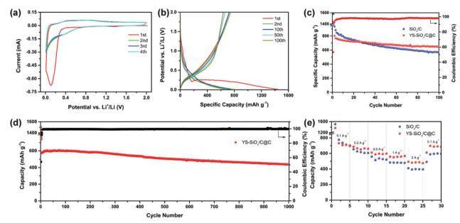
Fig. 5 CV curves (a) of YS-SiO<sub>x</sub>/C@C in the potential range of 0.01–2.0 V vs. Li<sup>+</sup>/Li at 0.1 mV s<sup>-1</sup>, selected galvanostatic charge–discharge profiles (b) of YS-SiO $_x$ /C@C at 100 mA g $^{-1}$ , cycling performances (c) of YS-SiO $_x$ /C@C and SiO $_x$ /C at 100 mA g $^{-1}$ , long-term cycling performances (d) of YS-SiO $_x$ /C@C at 500 mA  $g^{-1}$ , and rate performances (e) of YS-SiO<sub>x</sub>/C@C and SiO<sub>x</sub>/C
