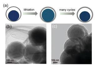
Fig. 6 Schematic illustration (a) showing the structure evolution of YS-SiO<sub>x</sub>/C@C during cycling, and TEM images (b and c) of YS-SiO<sub>x</sub>/C@C after 100 cycles at 2000 mA g<sup>-1</sup>.
