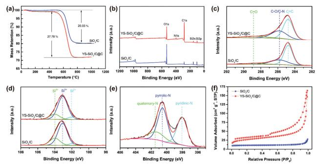
Fig. 4 TGA curves (a) of YS-SiO<sub>x</sub>/C@C and SiO<sub>x</sub>/C, XPS survey spectra (b), high-resolution C1s (c) and Si2p (d) spectra of YS-SiO<sub>x</sub>/C@C and SiO<sub>x</sub>/C, N1s (e) spectrum of YS-SiO $_x$ /C@C, and N $_2$  adsorption/desorption isotherms (f) of YS-SiO $_x$ /C@C and SiO $_x$ /C.
