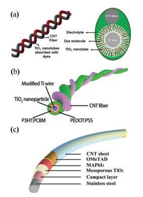
**Fig. 98** Fiber-shaped solar cells with different active materials and architectures. (a) Fiber-shaped dye-sensitized solar cell twisted from Ti wire and CNT fiber. (b) Fiber-shaped polymer solar cell with a twisted structure. (c) Fiber-shaped PVSC with a coaxial structure. Reproduced from ref. 712 with permission. Copyright (2016) Wiley-VCH.
