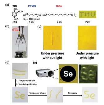
**Fig. 66** (a) Composition of the diselenide-bond-containing PU. (b) Material could bear 200 g weight after healing; the red part was stained with Nile red for clarity. (c) The crack disappeared after 24 h of light irradiation, demonstrating the healing property. (d) Typical shape-memory cycle of the material. (e) Material patterning achieved by a normal projector. Reprinted from ref. 503 and 504 with permission. Copyright (2015 and 2017) from Wiley-VCH and American Chemical Society.
