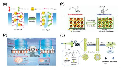
Fig. 90 (a) Direct blending of redox-responsive materials; (b) *in situ* crosslinking copolymerization of ion-exchange monomers; (c) *in situ* crosslinking copolymerization of salt-responsive monomers; (d) direct blending of amphiphilic polymers coupled with electrospinning technology. Adapted from ref. 635, 636, 638, and 639 with permission. Copyright (2015, 2016, 2017, and 2018) Elsevier Ltd, American Chemical Society, and Royal Society of Chemistry.
