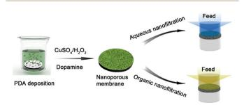
Fig. 91  $CuSO_4/H_2O_2$  triggered the rapid formation of PDA-based ultrathin selective layers with high uniformity and enhanced stability for both aqueous nanofiltration and organic nanofiltration. Reprinted from ref. 649 with permission. Copyright (2017) American Chemical Society.
