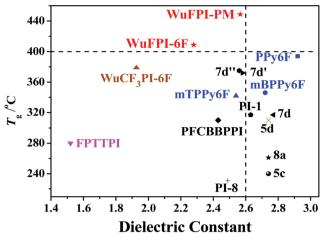
**Fig. 34** Relationship between k and  $T_g$  of the polyimides developed by Zhang's group and the reported intrinsic low-k polyimides. Reprinted from ref. 260 with permission. Copyright (2019) from Springer.
