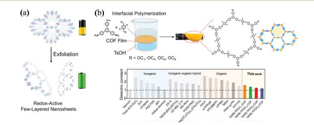
Fig. 101 (a) Schematic illustration for the exfoliation of 2D redox-active COFs into exfoliated COFs as cathodes for LIBs. (b) COF films prepared by interfacial polymerization, and their dielectric constants compared with those of typical commercial and representative ultralow-*k* materials. Adapted from ref. 725 and 726 with permission. Copyright (2017 and 2018) American Chemical Society and Wiley-VCH.
