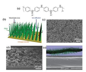
**Fig. 94** Application of conducting polymers in supercapacitors: (a) structure of PANI, (b) schematic mechanism of faster ion diffusion in nanowire arrays of PANI, (c) morphology of PANI nanowire array, (d) interconnected porous network of 3D graphene-based flexible film, and (e) schematic of the growth of PANI nanowires on CNT yarn and SEM image of actual yarn. Reproduced from ref. 683, 685 and 686 with permission. Copyright (2010 and 2013) American Chemical Society and Wiley-VCH.
