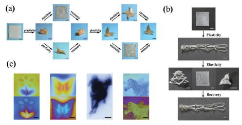
Fig. 82 Thermadapt SMP. (a) Origami-enabled shape memory; (b) kirigami-enabled shape memory; (c) digitally defined stress map visualized as the birefringent color under polarized light. Adapted from ref. 561, 562 and 563 with permission. Copyright (2016, 2016, and 2018) from Wiley-VCH, AAAS, and Nature Publishing Group.
