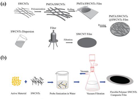
**Fig. 96** Schematic of fabricating a flexible electrode: (a) embedding a conventional cathode film into a CNT film acting as a flexible current collector and (b) fabrication of a free-standing film. Reprinted from ref. 689 and 697 with permission. Copyright (2015 and 2018) Wiley-VCH.
