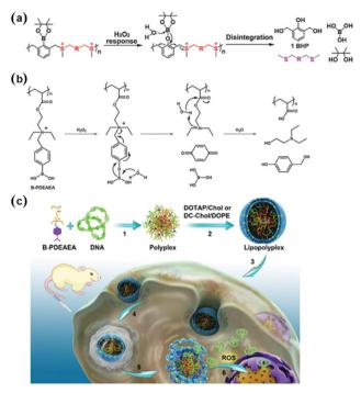
Fig. 53 (a and b) A positive-to-negative convention mechanism of surface charge for gene carriers. (c) Schematic representation of cationiclipid-coated ROS-responsive polyplexes for gene delivery. Reprinted from ref. 395, 396 and 399 with permission. Copyright (2017, 2016, and 2018) from Wiley-VCH and American Chemical Society.
