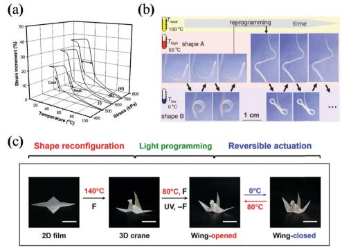
**Fig. 83** 2W-SME. (a) Quasi two-way shape-memory cycles under various constant stresses; (b) stress-free programmable two-way shape memory; (c) soft robot based on light-programmable two-way shape memory. Adapted from ref. 564, 565 and 587 with permission. Copyright (2008, 2013, and 2018) from American Chemical Society, Wiley-VCH, and AAAS.
