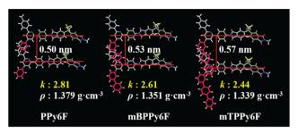
**Fig. 37** Intrinsic low-*k* polyimide containing the diphenylpyridine structure. Adapted from ref. 258 with permission. Copyright (2017) Royal Society of Chemistry.
