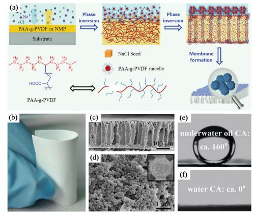
**Fig. 87** PAA-*g*-PVDF membrane with a micro-/nanohierarchical surface structure. (a) Schematic showing the fabrication of the membrane by a salt-induced phase-inversion process. (b) Photograph of the membrane. (c) Cross-section and (d) top-view SEM images of the membrane. Photographs of (e) an oil droplet on the membrane in water and (f) a water droplet on the membrane in air. Reproduced from ref. 624 with permission. Copyright (2014) Wiley-VCH.
