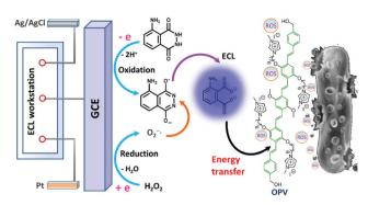
**Fig. 49** Schematic illustration of electricity-driven mechanism for ECL therapeutics to produce ROS and kill pathogenic bacteria. Ag/AgCl electrode: reference electrode; Pt electrode: counter electrode; glassy carbon electrode (GCE): working electrode. Reprinted from ref. 292 with permission. Copyright (2018) American Chemical Society.
