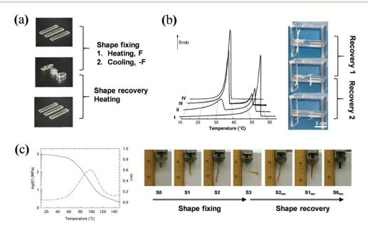
**Fig. 81** One-way SMEs. (a) dual-shape-memory cycle; (b) DSC curves for polymers with two distinct phase transitions and the associated triple-shapememory recovery; (c) DMA curve for a polymer with a single broad transition and the associated multishape-memory cycle. Adapted from ref. 17, 558 and 559 with permission. Copyright (2015, 2006, and 2010) from Elsevier Ltd., National Academy of Sciences, U.S.A., and Nature Publishing Group.
