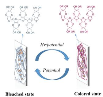
**Fig. 75** Trifunctional CdSe quantum dots–polymer composite film with electrochromic, electrofluorescent, and light-induced coloration effects. Adapted from ref. 543 with permission. Copyright (2018) from Elsevier Ltd.
