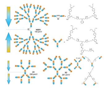
**Fig. 41** Chemical structures of the high-generation dendrimer HGD1 and X1 and X2 with a Janus structure.
