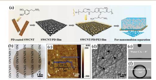
**Fig. 88** SWCNT/PD/PEI composite membrane. (a) Schematic showing the fabrication of a membrane and the separation of oil-in-water nanoemulsion. (b) Digital photograph of a free-standing membrane. (c) AFM image and height profile of the membrane. (d) TEM image of the membrane. Photographs of (e) a water droplet on the membrane in air and (f) an oil droplet on the membrane underwater. Reproduced from ref. 628 with permission. Copyright (2015) Royal Society of Chemistry.
