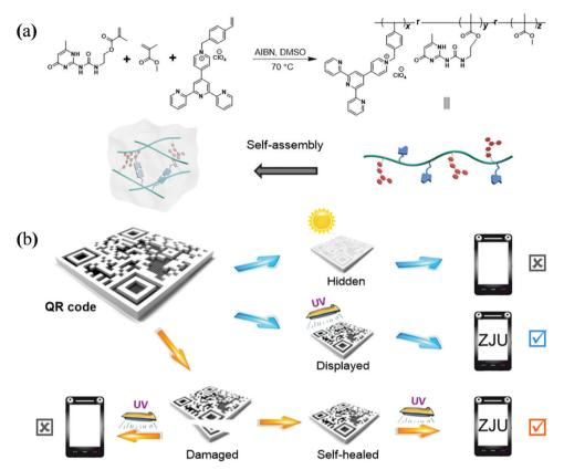
**Fig. 64** (a) Synthesis of the polymer and its self-assembly in solution to form a white-light-emitting fluorescent SP gel *via* intermolecular hydrogen bonding. (b) Schematic representation of data recording, data security protection, and data recovery of a quick response code constructed using this gel. Adapted from ref. 494 with permission. Copyright (2017) Royal Society of Chemistry.
