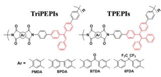
**Fig. 35** Low-*k* polyimides containing triphenylethylene and TPE moieties. Adapted from ref. 255 and 256 with permission. Copyright (2012 and 2013) American Chemical Society and Wiley-VCH.
