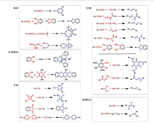
Fig. 99 Chemical reactions for the preparation of COFs.
