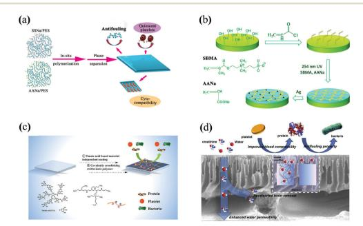
**Fig. 89** (a) *In situ* crosslinking polymerization of monomers; (b) *in situ* crosslinking polymerization combined with post-crosslinking of monomers; (c) surface coating followed by *in situ* crosslinking of polymers; (d) direct blending of nanofibers and nanotubes. Adapted from ref. 631–634 with permission. Copyright (2016, 2017, 2018, and 2017) Elsevier Ltd and American Chemical Society.
