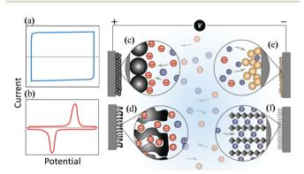
**Fig. 93** Typical CV curves of a (a) supercapacitor and (b) battery, and the charge storage mechanism for different materials: (c) surface charge accumulation in carbon and (d) porous carbon; pseudocapacitive behavior for (e) redox reaction and (f) ion intercalation. Reprinted from ref. 669 with permission. Copyright (2014) from AAAS.
