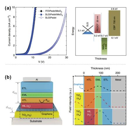
Fig. 18 (a) Energy level diagram of the single-layer graphene (SLG) anode/PEDOT:PSS/MoO<sub>3</sub>/CBP structure. Reproduced with permission from ref. 208. Copyright 2013 Macmillan Publishers Limited. (b) Schematic device structure of the proposed OLEDs and electromagnetic field intensity distribution (dashed lines) of the OLEDs under study for their respective first-order cavity design. Reproduced with permission from ref. 209. Copyright 2016 Macmillan Publishers Limited.
