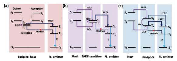
Fig. 6 Schematic diagrams of sensitized fluorescent OLEDs. (a) Exciplex sensitized FOLEDs, (b) TADF sensitized FOLEDs and (c) phosphor sensitized FOLEDs.
