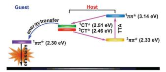
Fig. 2 The schematic energy transfer routes of the TTA process. Reproduced with permission from ref. 21. Copyright 2014 The Royal Society of
