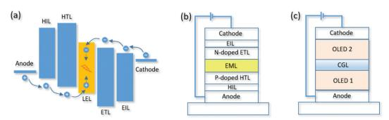
Fig. 4 Representative device architectures of OLEDs. (a) The working mechanism of OLEDs, (b) charge injection and transport in OLEDs enhanced by p- and n-type electrical doping, and (c) tandem OLED structures with stacked emission units connected by a charge generation layer (CGL).
