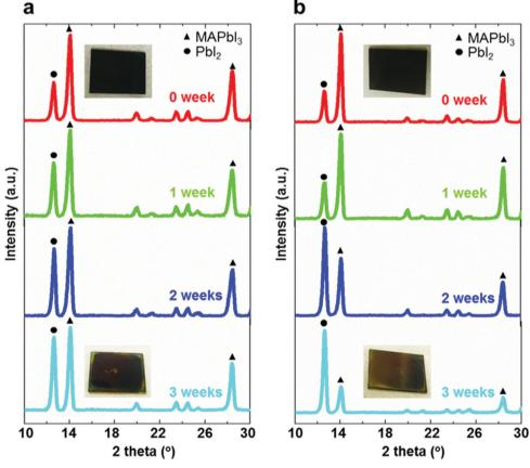
Fig. 3 XRD spectra in the  $2\theta$  range from  $10^{\circ}$  to  $30^{\circ}$  of the perovskite films based on (a) the bilayer mesoporous scaffold and (b) the single mesoporous scaffold after different aging times in ambient air at >65% relative humidity. The insets are the top views of the corresponding perovskite films.
