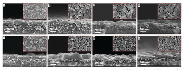
Fig. 4 SEM images of the perovskite film generated on the bilayer mesoporous scaffold after aging for (a) 0 week, (b) 1 week, (c) 2 weeks and (d) 3 weeks; SEM images of the perovskite film generated on the single mesoporous scaffold after aging for (e) 0 week, (f) 1 week, (g) 2 weeks and (h) 3 weeks. All aging tests were carried out in ambient air at >65% relative humidity. The insets are the top views of the corresponding perovskite films.
