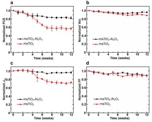
Fig. 2 Evolution of photovoltaic parameters: (a) PCE, (b)  $V_{oc}$ , (c)  $J_{sc}$ , and (d) FF of the PSCs based on different mesoporous scaffolds stored in ambient air at >65% relative humidity. The measurement was carried out immediately after fabrication and once a week in the following 12 weeks. Each value is the average over 8 cells in the same counterparts.
