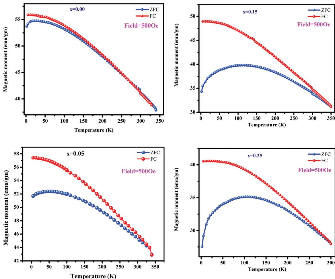
Fig. 10 FC–ZFC curves for  $\text{Ni}_{0.70-x}\text{Cu}_x\text{Zn}_{0.30}\text{Fe}_2\text{O}_4$  ( $x = 0.00, 0.05, 0.15, \text{ and } 0.25$ ).
