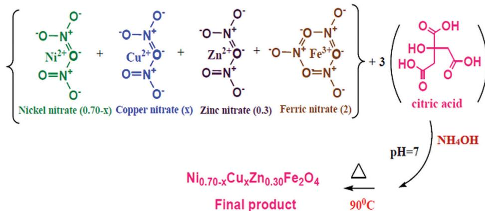
Fig. 2 Schematic of the mechanism of the  $\text{Ni}_{0.70-x}\text{Cu}_x\text{Zn}_{0.30}\text{Fe}_2\text{O}_4$  ( $x = 0.00, 0.05, 0.15, \text{ and } 0.25$ ) synthesis.
