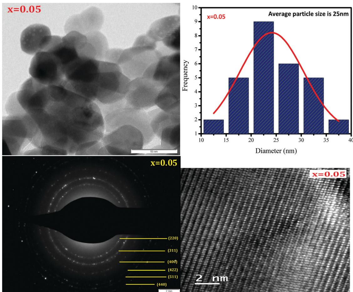
Fig. 5 TEM image, particle size distribution, SAED pattern, and HR-TEM image of Ni<sub>0.70-x</sub>Cu<sub>x</sub>Zn<sub>0.30</sub>Fe<sub>2</sub>O<sub>4</sub> (x = 0.05).
