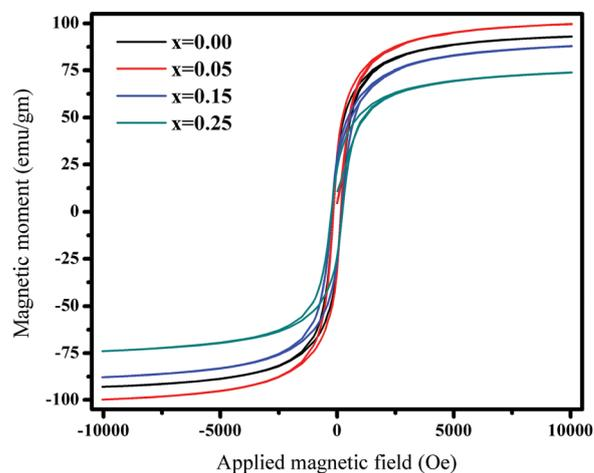
Fig. 8  $M-H$  plots for  $\text{Ni}_{0.70-x}\text{Cu}_x\text{Zn}_{0.30}\text{Fe}_2\text{O}_4$  ( $x = 0.00, 0.05, 0.15,$  and  $0.25$ ) obtained at 5 K.
