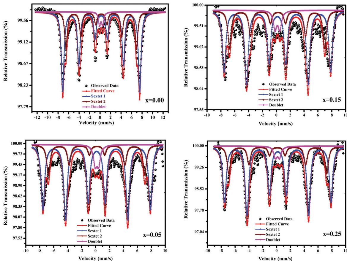
**Fig. 11** Mössbauer spectra of Ni<sub>0.70-x</sub>Cu<sub>x</sub>Zn<sub>0.30</sub>Fe<sub>2</sub>O<sub>4</sub> ( $x = 0.00, 0.05, 0.15,$  and  $0.25$ ).
