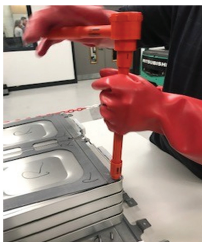
Fig. 5 (a) Pouch cell tabs ultrasonically welded to copper busbar, (b) module interconnections utilising threaded bolts through solid busbars (c) dismantling of pack sub-assemblies using standard shop tooling – all Nissan Leaf 1 st generation.
