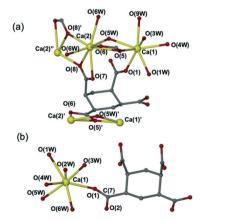
Fig. 4 Crystal structures of (a)  $[Ca_2(C_{10}H_8O_8)(H_2O)_7]\cdot 2H_2O$  (8) and (b)  $[Ca(C_{10}H_{10}O_8)(H_2O)_6]\cdot H_2O$  (9).
