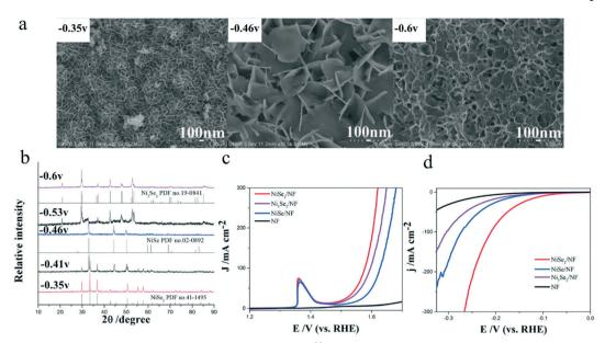
Fig. 3 Controlled synthesis of nickel selenides in different crystal phases.<sup>22</sup> (a) FESEM images of the as-prepared nickel selenides with different crystal phases taken at various deposition potentials: -0.35, -0.46, and -0.60 V; (b) XRD patterns of the nickel selenides; (c and d) polarization curves of these nickel selenides for (c) HER and (d) OER.
