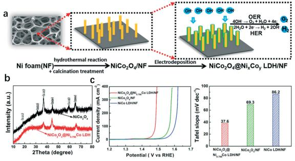
Fig. 2 Hybrid catalyst NiCo<sub>2</sub>O<sub>4</sub>@Ni<sub>x</sub>Co<sub>v</sub> LDH/NF with amorphous Ni<sub>x</sub>Co<sub>v</sub> LDH and crystallized NiCo<sub>2</sub>O<sub>4</sub> as the shell and core, respectively.<sup>37</sup> (a) Illustration of the fabrication process of the hybrid catalyst, (b) XRD of  $NiCo_2O_4$  and  $NiCo_2O_4$  and Nslopes of NiCo<sub>2</sub>O<sub>4</sub>@Ni<sub>0.796</sub>Co LDH/NF, NiCo LDH/NF, and NiCo<sub>2</sub>O<sub>4</sub>/NF.
