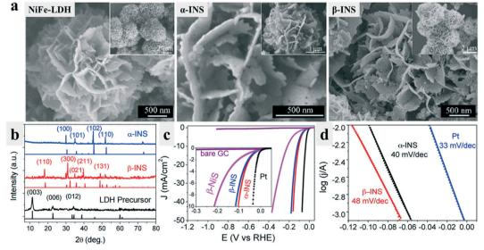
Fig. 4 Morphology retained phase-conversion from LDH to  $\beta$ -INS and  $\alpha$ -INS sulfides. <sup>23</sup> (a) SEM images of the FeNi LDH precursor,  $\beta$ -INS nanosheets, and metallic  $\alpha$ -INS nanosheets. (b) XRD pattern of the LDH precursor,  $\beta$ -INS and  $\alpha$ -INS. (c) Linear sweep voltammetry (LSV) curves of the  $\beta$ -NIS,  $\beta$ -INS, and  $\alpha$ -INS catalyzed HER. (d) Tafel plots of the Pt,  $\beta$ -INS, and  $\alpha$ -INS catalyzed HER.
