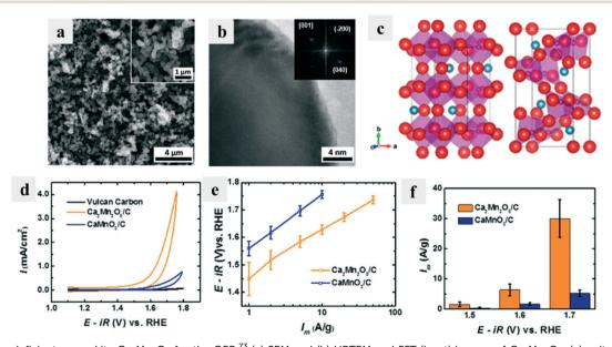
Fig. 8 Oxygen-deficient perovskite  $Ca_2Mn_2O_5$  for the OER. <sup>73</sup> (a) SEM and (b) HRTEM and FFT (inset) images of  $Ca_2Mn_2O_5$ ; (c) unit cell structures of  $CaMnO_3$  (left) and  $Ca_2Mn_2O_5$  (right); (d) iR-corrected data of  $Ca_2Mn_2O_5/C$ ,  $CaMnO_3/C$ , and Vulcan carbon XC-72; (e) Tafel plot of mass activities; (f) mass activities at various applied potentials.
