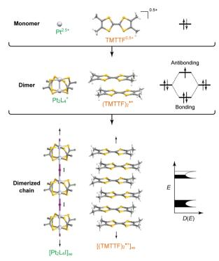
Fig. 1 Comparison of the monomeric, dimeric, and assembled structures of (left)  $Pt_2L_4I$  (L =  $RCS_2^-$ ) and (right) (TMTTF)<sub>2</sub>X (X: monoanion) together with their electronic states (D(E): density of states).
