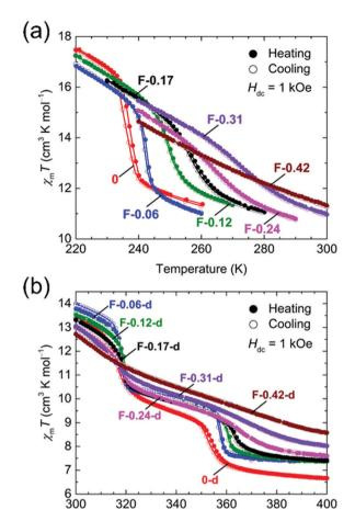
Fig. 3 Temperature dependence of  $\chi_m T$  for F-Y (a) and F-Y-d (b) measured at  $H_{\rm dc}=1$  kOe ( $\chi_m=M_m/H_{\rm dc}$ ), where narrow temperature ranges of 220–300 K and 300–400 K, respectively, were used.
