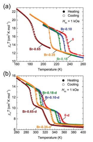
Fig. 2 Temperature dependence of  $\chi_m T$  for **Br-Y** (a) and **Br-Y-d** (b) measured at  $H_{\rm dc}=1$  kOe ( $\chi_{\rm m}=M_{\rm m}/H_{\rm dc}$ ), where the narrow temperature ranges of 160–260 K and 260–400 K, respectively, were used.
