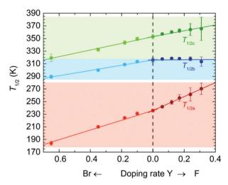
**Fig. 4** Variations of the  $T_{1/2}$  value of TDETs for the site-doped rate Y in the solid solution series of **X-Y** and **X-Y-d**, whereas the basis of Y = 0 corresponded to **0** and **0-d**. The left and right scales represent **Br-Y/Br-Y-d** and **F-Y/F-Y-d**, respectively. The solid lines are least-square linear fitting lines for the respective series.
