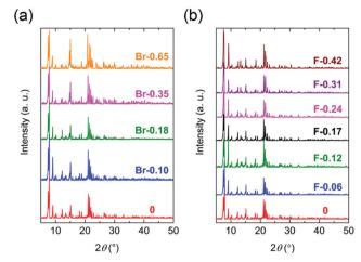
Fig. 1 PXRD patterns of Br-Y (a) and F-Y (b) measured at room temperature
