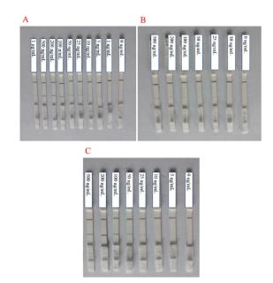
Fig. 3 Au NP based LFITS for STX2 sensitivity detection by using different NC membranes: (A) Sartorius CN95, (B) Sartorius CN140, and (C) Vivid 170.
