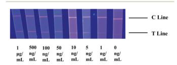
Fig. 5 CdTe QD based LFITS for STX2 sensitivity detection.
