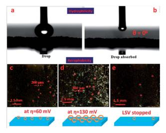
Fig. 6 Wettability test of the Cuf@Ni<sub>5</sub>P<sub>4</sub> surface: (a) before; and (b) after placing a liquid drop with a contact angle of 0°. (c-e) Optical images with a schematic diagram in the bottom panel showing the bubble formation behavior on the Cuf@Ni<sub>5</sub>P<sub>4</sub> surface at different overpotentials and at the end of LSV.
