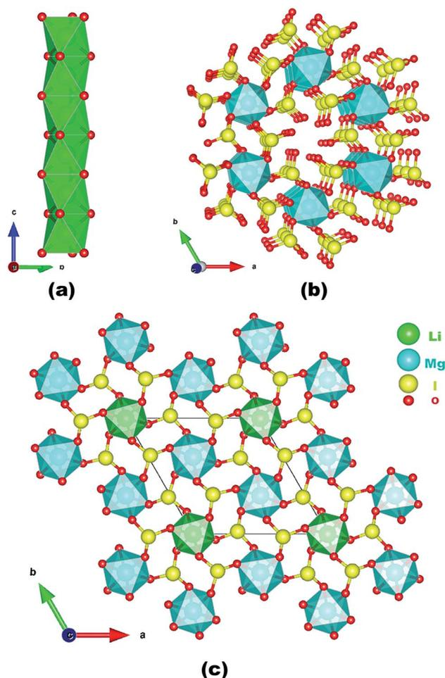
Fig. 1 A 1D chain of face-sharing  $\text{LiO}_6$  octahedra along the  $c$ -axis (a); the 3D  $[\text{Mg}(\text{IO}_3)_6]^{4-}$  anionic framework along the  $c$ -axis (b); and the view of the structure of LMIO along the  $c$ -axis (c).
