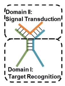
Scheme 1 Structure illustration of a TWJ-based DNA molecular switch. Domains I and II are responsible for target recognition and signal transduction, respectively. Domain I can be functional nucleic acids such as aptamers.
