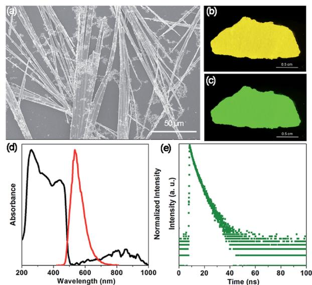
Fig. 2 (a) SEM image of the 1D OIHP-AD micro-belts. Photographs of the self-supporting OIHP-AD film (about  $0.8 \times 3 \text{ cm}^2$ ) under (b) daylight and (c) UV (365 nm). (d) UV-vis-NIR absorption (black) and fluorescence emission spectra (red, excitation at 400 nm) of OIHP-AD in the solid state at room temperature. (e) Time-resolved fluorescence decay of OIHP-AD in the solid state.
