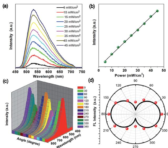
Fig. 6 (a) Up-conversion fluorescence spectra of OIHP-AD excited using an 800 nm laser under different pump powers. (b) The changes in intensity with increasing pump powers. (c) Polarized fluorescence spectrum of OIHP-AD at various angles (0–360°). (d) Fluorescence intensity of the OIHP-AD as a function of the polarizer rotation angle.
