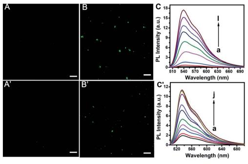
Fig. 6 Fluorescence images of TOTO-1 in the absence and presence of telomerase (7500 cells per mL) (A and B) and PARP-1 (0.8 U/20 μL) (A' and B'). The scale bar is 5 μm. Fluorescence spectra of the detection system with increasing concentration of telomerase from 2 to 4000 A549 cells per mL (C) and PARP-1 from 0.02 U to 1.5 U (C').
