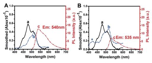
Fig. 3 Absorption spectra of free TOTO-1 (a in A and B) and TOTO-1 in the presence of G-rich extended primer (b, A) and PAR (b, B). Fluorescence spectra of TOTO-1 in the presence of G-rich extended primer (c, A) and PAR (c, B).
