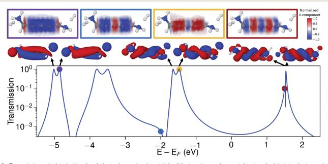
Fig. 8 Transmission calculated with s-band electrodes, molecular orbitals of the junction, and current density calculated at select energies for the (-)S(-) conformation of S-1,5-diamino-[4] cumulene. The current density vector field is shown on a high-density grid and is colored by the  $\theta$ -component. In the transmission plot, arrows indicate orbital energy (at the corresponding transmission resonances), colored dots indicate the energy at which the current density is calculated.
