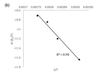
Fig. 3 (a) Modelled (Copasi) reaction network for the reaction of 1 with allyl benzene. (b) Eyring analysis plot of  $ln(k_2/T)$  versus 1/T.
