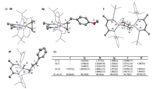
Fig. 2 (a) Solid state structures of 2b, 2g, 3 and 4f. (b) Comparison of bond lengths (Å) and angles (°).
