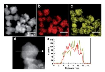
Fig. 3 Scanning transmission electron microscopy images of  $Au_{0.5}Ir_{0.5}$  NPs. (a) a HAADF-STEM image. (b), (c) Au-M and Ir-M STEM-EDX maps (red, Au; yellow, Ir). (e) Compositional line profiles of Au (red) and Ir (dark yellow) for the  $Au_{0.5}Ir_{0.5}$  nanoparticle recorded along the arrow shown in (d) the HAADF-STEM image.
