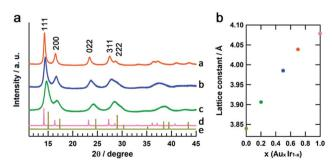
Fig. 4 X-ray diffraction analysis of  $Au_xIr_{1-x}$  NPs. (a) Powder XRD patterns of a;  $Au_{0.7}Ir_{0.3}$  NPs, b;  $Au_{0.5}Ir_{0.5}$  NPs, c;  $Au_{0.2}Ir_{0.8}$  NPs, d; Au and e; Ir powders. (b) A plot of the changes in the lattice constants verses the metal composition.
