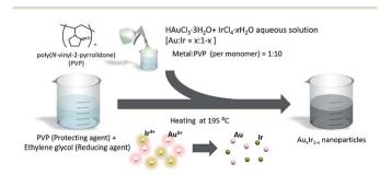
Fig. 2 Schematic image of the synthesis of  $\mathrm{Au_xIr}_{1-x}$  solid-solution alloy NPs.
