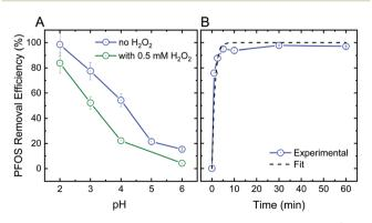
Fig. 3 (A) Effect of pH on the adsorption efficiency of 1 mg  $L^{-1}$  perfluorooctanesulfonic acid (PFOS) by 1 mg mL<sup>-1</sup> ceria nanoparticles after 1 hour of mixing in the absence (blue) and presence (green) of 0.5 mM H<sub>2</sub>O<sub>2</sub>. (B) PFOS adsorption kinetics and best-fit line (pseudofirst order) at pH 2.
