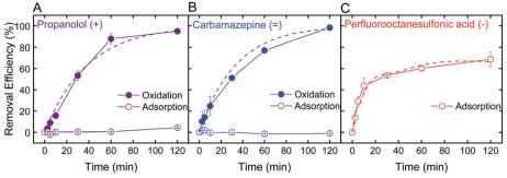
Fig. 4 Removal kinetics and best-fit line (pseudo-first order) of 1 mg  $L^{-1}$  (A) propranolol (purple), (B) carbamazepine (blue), and (C) per-fluorooctanesulfonic acid (red) by electrospun ceria/silica nanofiber composites for a final concentration of 1 mg nanoceria per mL of treated solution, through oxidation (solid circles) at pH 2 in 0.5 mM  $H_2O_2$  and adsorption (open circles) at pH 2 and no  $H_2O_2$ .
