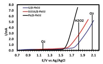
Fig. 3 LSV grame of  $\beta$ -PbO<sub>2</sub> electrodes in Na<sub>2</sub>SO<sub>4</sub> (0.25 M) at pH = 6.0. Scan rate = 100 mV s<sup>-1</sup>.
