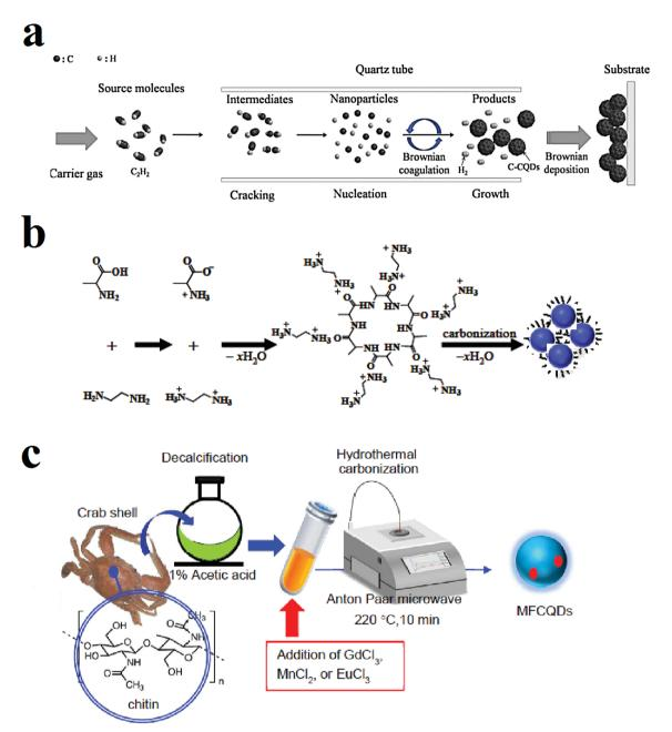
Fig. 2 (a) Synthesis of CQDs through CVD method using  $C_2H_2$  as the carbon source, reprinted with permission from ref. 47, copyright 2016 Elsevier Ltd., (b) synthesis of the CQDs through the hydrothermal method using alanine and ethylenediamine, reprinted with permission from ref. 66, copyright 2015 Elsevier Ltd., (c) microwave-assisted pyrolysis synthesis of magnetofluorescent CQDs from crab shell, reprinted with permission from ref. 81, copyright 2017 American Chemical Society.
