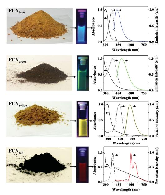
Fig. 6 Different CQDs synthesized through different controlled carbohydrate carbonization methods, the solution containing CQDs and regarding absorption (solid line), excitation (dashed line) and emission (colored line) spectra; the emission spectra are recorded by excitation at 370 nm for blue CQDs, at 400 nm for green CQDs, at 425 nm for yellow CQDs, and at 385 nm for red CQDs, reprinted with permission from ref. 155, copyright 2013 Springer Nature.
