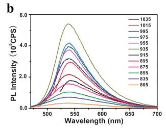
Fig. 4 Excitation and emission spectra of the CQDs that were synthesized *via* heating of the ascorbic acid aqueous solution; (a) emission spectra at excitations ranging from 290 nm to 500 nm, (b) upconversion seen in the emission spectra of the CQDs, the PL emission spectra for excitations from 805 nm to 1035 nm, reprinted with permission from ref. 152, copyright 2012 Royal Society of Chemistry.
