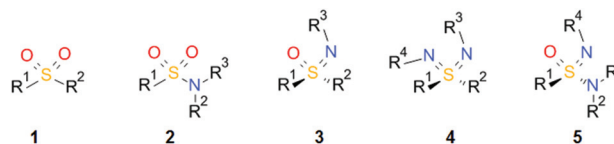
Scheme 1 General structures of sulfones 1 , sulfonamides 2 , and aza analogues sulfoximines 3 , sulfondiimines 4 and sulfonimidamides 5 .
