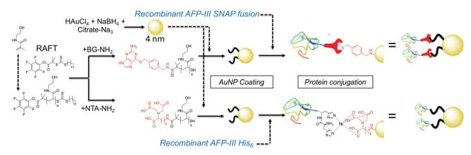
Fig. 1 Synthesis of gold/polymer/antifreeze protein hybrid particles. NTA = Nitrilotriacetic acid;  $BG = O^6$ -benzylguanine;  $His_6$  = hexa-histidine tag. Red 'wrench' represents the SNAP-tag.
