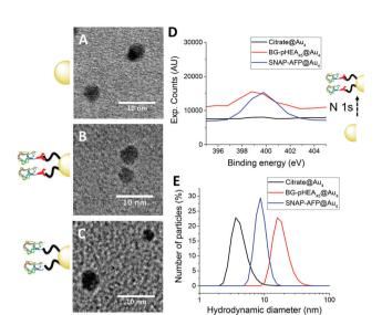
Fig. 3 Nanoparticle characterization. (A–C) Transmission electron micrographs of citrate@Au $_4$ , SNAP-AFP-BG-pHEA $_4$ 5@Au $_4$  and His-AFP-Ni-NTA-pHEA $_{17}$ @Au $_4$  respectively; (D) N 1s peak from XPS upon conjugation of SNAP-AFP; (E) diameter from dynamic light scattering.
