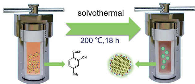
Fig. 1 Schematic illustration of the preparation of N-CD nanomaterials.
