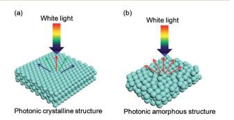
Fig. 1 Typical photonic nanostructures of colloidal assembled structural color: (a) highly ordered PCSs generating iridescence; (b) short-ordered PASs exhibiting non-iridescence.
