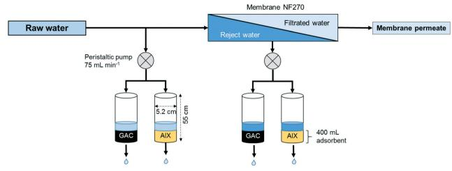
Fig. 1 Schematic of the treatment of PFAS contaminated raw water using two nanofiltration membranes connected in series resulting in filtrated water and membrane reject water. In addition, the raw water and the membrane reject water were treated using granulated activated carbon (GAC) or anion exchange (AIX) adsorption material.
