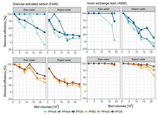
Fig. 2 Removal efficiency [%] of frequently detected PFCAs (top) and PFSAs (bottom) for the evaluated granular activated carbon material (F400, left) and anion exchange resin (A600, right) depending on bed volumes treated. Treatment of both raw water and water rejected by a NF270 membrane was evaluated. Please note that lines are solely added to guide the eye, and do not represent a model.
