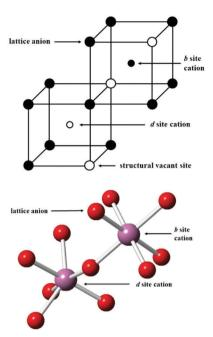
Fig. 1 Lattice sites in In<sub>2</sub>O<sub>3</sub>. In the bottom figure, the coordination of the cations is shown, with indium ions represented by larger purple spheres and oxygen ions by smaller red spheres.
