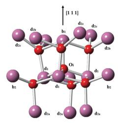
Fig. 3 Interstitial oxygen in In<sub>2</sub>O<sub>3</sub>. In ions are represented by larger purple spheres while O ions are represented by smaller red spheres.
