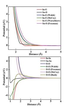
Fig. 2 Interatomic potential model for  $\rm In_2O_3$  and  $\rm SnO_2$ . Metal-oxygen interactions are shown in the top panel, while metal-metal and oxygen-oxygen interactions are shown in the bottom panel. Our model is compared with other previously published ones (see the text for details).
