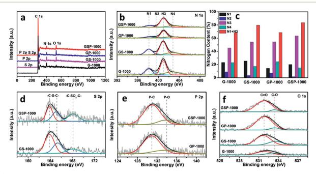
Fig. 3 (a) XPS survey spectra. (b) High resolution N 1s XPS spectra. (c) The content percentages of different nitrogen species. (d) High resolution S 2p XPS spectra. (e) High resolution P 2p XPS spectra. (f) High resolution O 1s XPS spectra.
