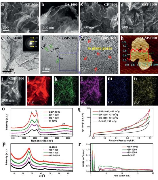
Fig. 2 (a-d) SEM images of G-1000, GS-1000, GP-1000 and GSP-1000, showing a 2D sheet-like morphology. (e-g) TEM and HRTEM images of GSP-1000; inset of (e) shows the SAED pattern. (h) AFM image and height profile of GSP-1000. (i-n) HAADF-STEM image of GSP-1000 and the corresponding EDX elemental maps of C, N, P, S, and O. (o) Raman spectra, (p) XRD patterns, (q) nitrogen adsorption/desorption isotherms and (r) pore size distributions (PSDs) of the sample series.
