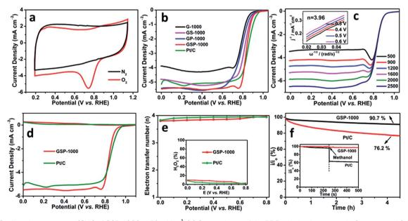
Fig. 4 (a) Cyclic voltammograms (CVs) of GSP-1000 at 50 mV s<sup>-1</sup>. (b) Comparisons of the RDE polarization curves in  $O_2$ -saturated 0.1 M KOH at 1600 rpm with 10 mV s<sup>-1</sup>. (c) RDE polarization curves of GSP-1000 at different rotation speeds. (d) RRDE curves at 1600 rpm. (e) The corresponding electron transfer numbers; inset: peroxide percentages. (f) i-t Response at 0.8 V (vs. RHE) at 1600 rpm; inset shows the methanol crossover effect test upon addition of 1 M methanol
